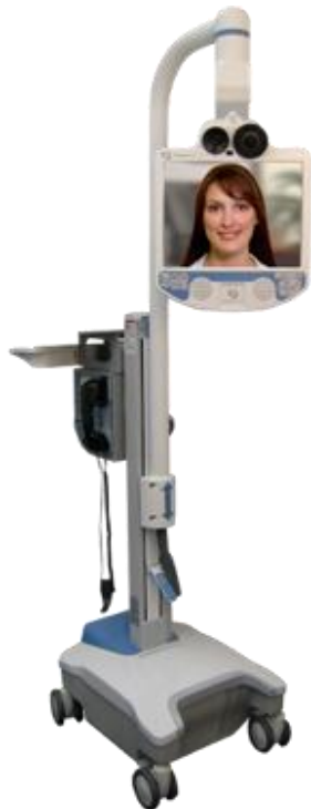
Figure 8. Intouch RP-Lite Robot allows stroke neurologist to remotely assess the patient via the use of telemedicine technology in the form of high-quality videoconferencing (HQ-VTC).
